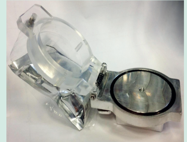
Large box within vacuum, almost final design, capacity for 4 stubs
