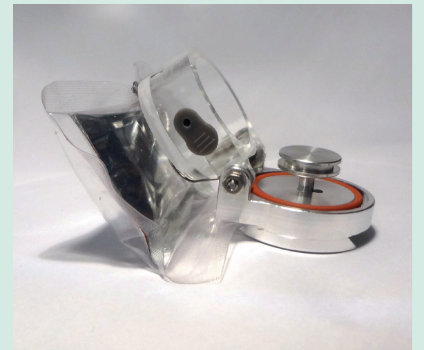
Small box within vacuum, capacity for one standard stub
